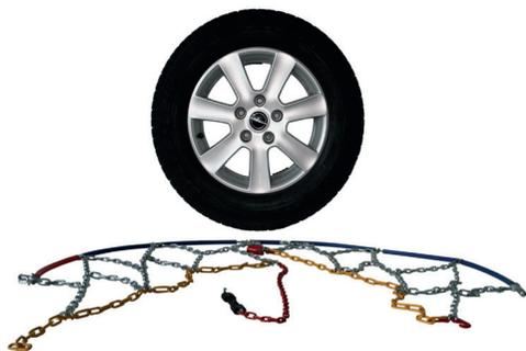
1. Unfold the chain on the ground, with the yellow plastic end of the cable towards the left.
