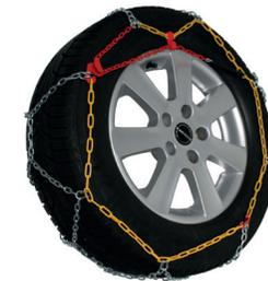
8. Thread the elastic tensioner into the red metal ring, and then by pulling it as much as possible. Fasten the elastic tensioner into a link of the side chain.
