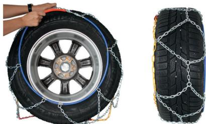
5. Push the flexible cable towards the interior of the wheel and make sure it is not on the tyre tread.
