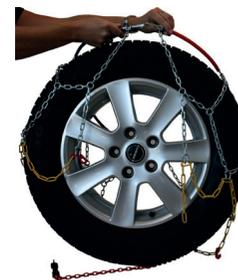
3. Pull upwards the flexible cable so that the two steel ends can be fastened together.
