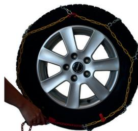
6. Pass the red chain into the red self-locking slide gear.
