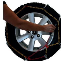
7. Pass the red chain into the red self-locking slide gear.
